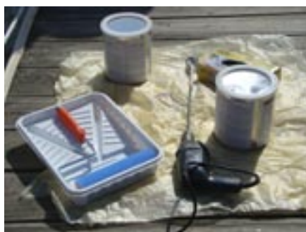
Ultra Tuff non-skid contains suspended particles of rubber. To keep them properly mixed, Chuck stirred the product regularly with an electric drill accessory.
