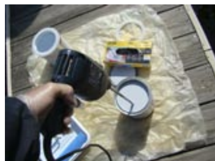
Ultra Tuff non-skid contains suspended particles of rubber. To keep them properly mixed, Chuck stirred the product regularly with an electric drill accessory.
