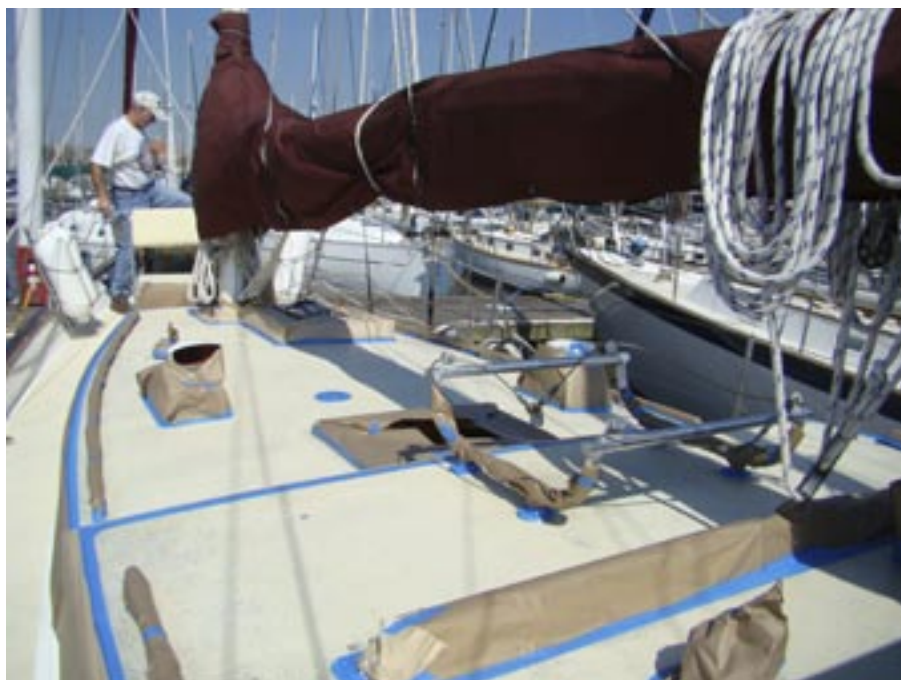
After removing from the deck whatever fittings they reasonably could, Chuck and Susan taped around what remained, above, then added masking paper as further protection, right.
